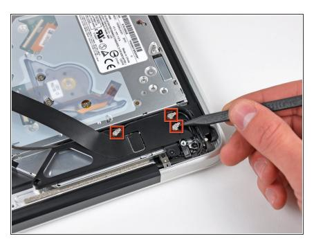
Use the tip of a spudger to pry the three antenna connectors up off the AirPort/Bluetooth board.
