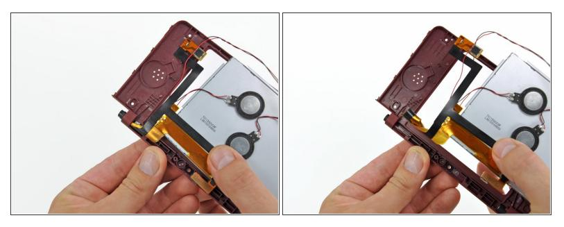
Holding the upper LCD and the cameras together, pull the cables through the hinge in the front bezel.
