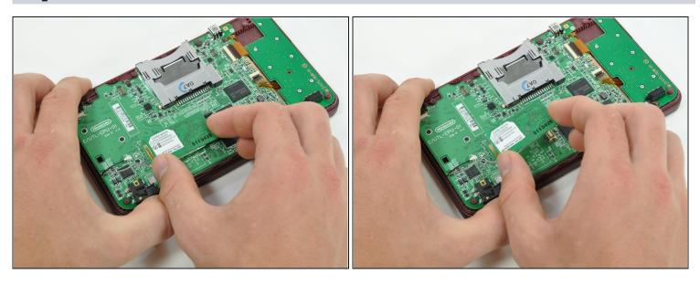
• Lift the Wi-Fi board up off its socket on the motherboard.
