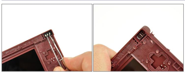
• Using a pair of tweezers, remove the LED diffuser bracket and the LED diffuser from the upper case of the DSi XL.
