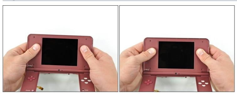
• Using two hands, gently slide the rear bezel upwards.
