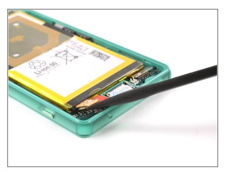
Disconnect the battery flex cable.
