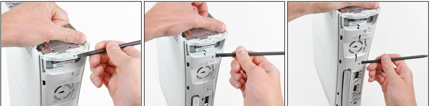
ⓘ The upper and lower cases are attached via several latches, located in the front and back of the console. These latches must be disengaged to separate the upper case from the console.
