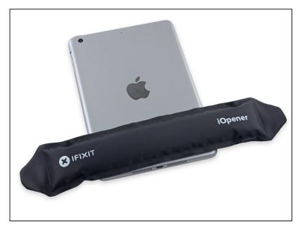
Place a heated iOpener on the bottom of the rear case for one minute.
