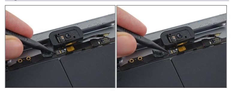
• Use the tip of a spudger to gently lift the tab on the microphone ribbon cable's ZIF connector.
