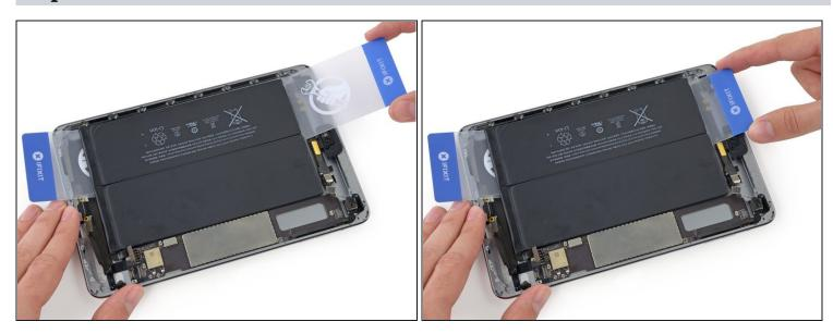
• Insert the second card under the battery near the headphone jack.
