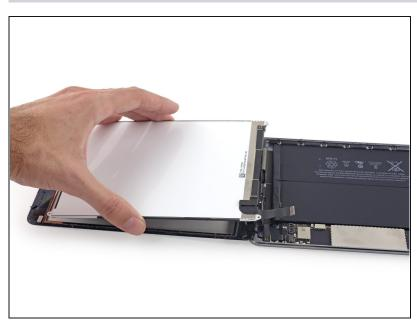
• Lift and remove the LCD from the iPad Mini 3.
