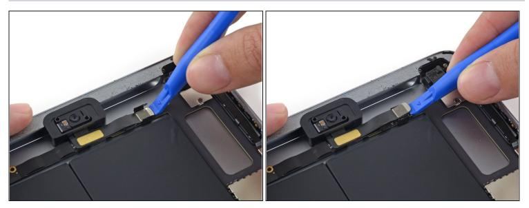
• Use a plastic opening tool to lift the front-facing camera cable connector straight up off of its socket on the logic board.
