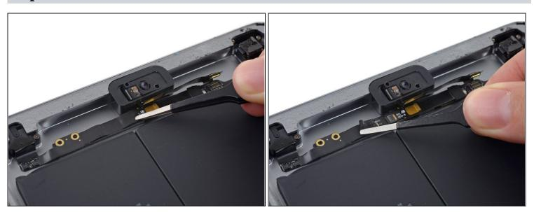
• Use a set of tweezers to peel up the small piece of tape covering the microphone cable connector.
