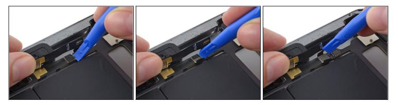
• Use a plastic opening tool to fold the headphone jack cable clips outward, away from the cable, freeing the cable connector.
