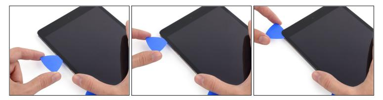
• Slide the opening pick around the top left corner of the iPad to separate the adhesive.
