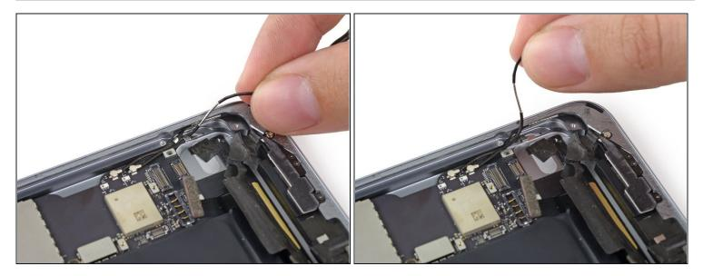
• De-route the antenna cable from the retaining clip.
