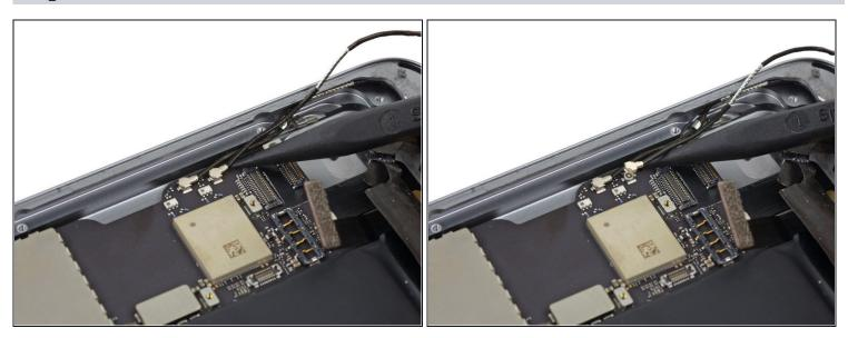
• Use the point of a spudger to lift the left antenna cable connector straight up off of its socket on the logic board.
