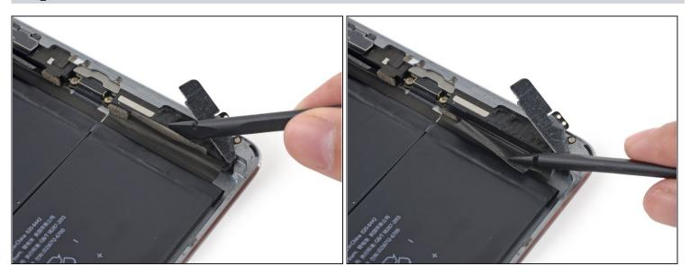
• Use the flat end of a spudger to fold the wide left-hand piece of tape away from the left speaker.
