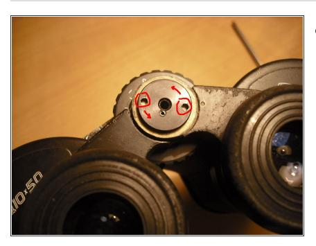
Insert pointy-nose pliers into both holes. Turn anticlockwise.
