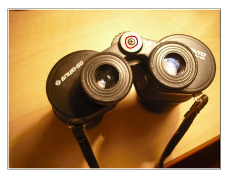
Turn cross head screwdriver anticlockwise.
