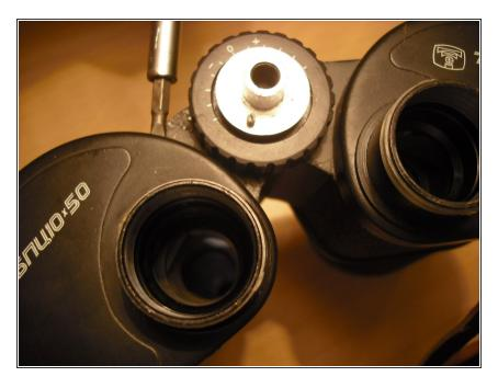
There are no screws holding the dust cover on but you will need to unscrew and remove each eyepiece barrel (not shown in photo). The cover should then lift off fairly easily. If not then work around it with a screwdriver. Eventually it will come off.
