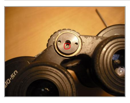
Turn CR-V 1.0 screw bit anticlockwise. Because this screw is so small, it may help to magnitise your screw bit by brushing it with a magnetic screwdriver first. This will make the screw stick to the screw bit. Have a dish handy to keep the tiny screw in.
