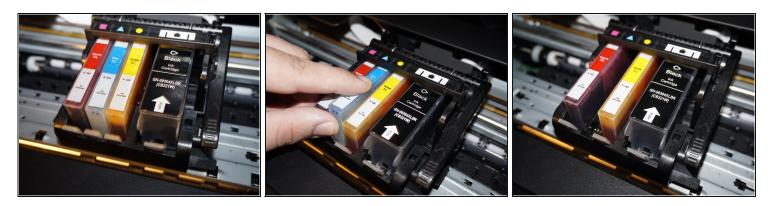
Remove the ink cartridges from the printer. Install the shipping caps or put them in a plastic bag.
