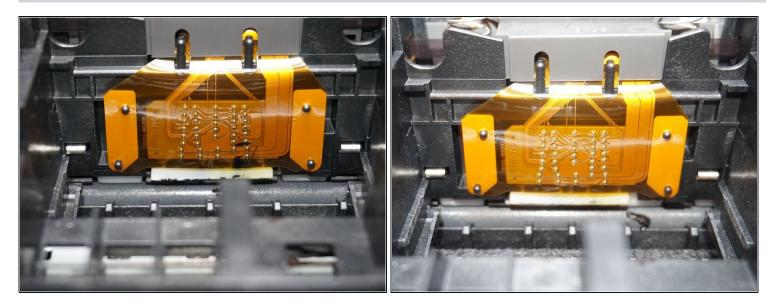
⚠ Failure to clean this area may result in a Ink System Failure warning, and a lost calibration.
