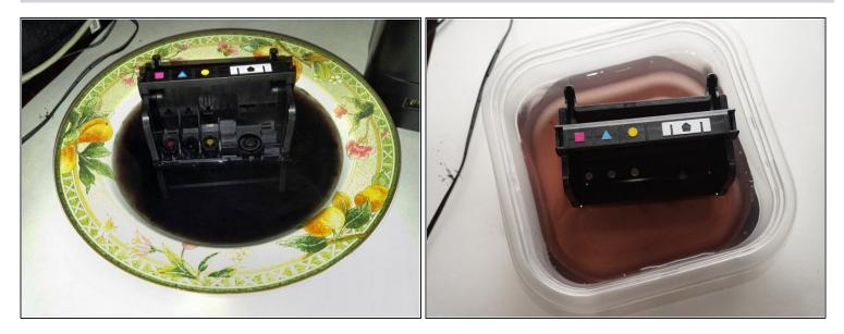
⚠ Only use alcohol as a final option. It may damage the printhead seals! IF USED, FLUSH WITH CLEAN WATER 3 TIMES.
