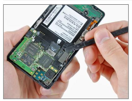
Disconnect the display ribbon connector from its socket on the motherboard using the flat end of a spudger.
