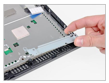
Remove the control board bracket.
