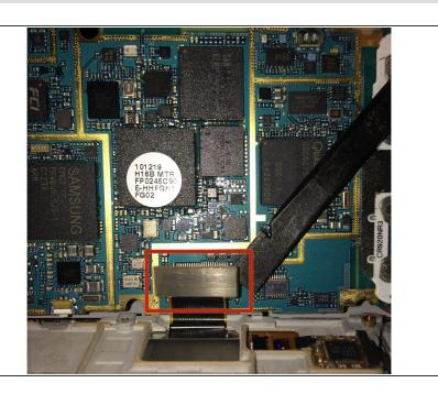
Using your spudger/plastic pry tool, disconnect the LCD/Digitizer flex cable.
