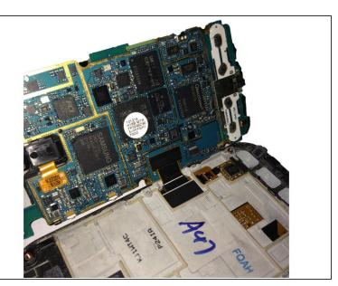
After removing both flex cables, slowly move the logic board to the left of the screen assembly.
