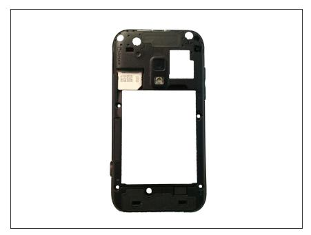
Lift the rear housing from the display assembly.
