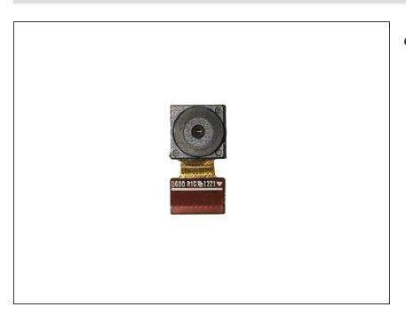
Carefully pull the camera out of it's connector and set to the side.
