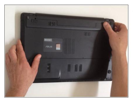
Switch off the laptop and remove the battery.
