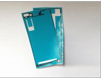
Before installing the new cover, you must clean the phone from the old adhesive tape and install a new one (if your spare part has come without double sided adhesive tape).
