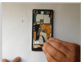
Unscrew the screw and remove the Wi-Fi Antenna.
