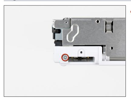
Remove the 8.2 mm Tri-Point screw that was hidden beneath the battery door.
