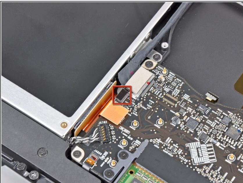
ⓘ Before disconnecting the camera cable, a small plastic retainer stuck to the logic board must first be moved out of the way.
