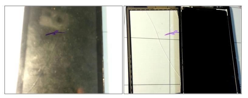
To separate glass (with touch) just heat it up to loosen adhesive
