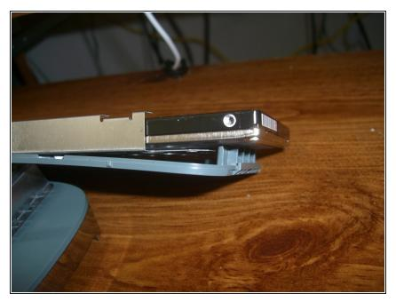
To actually get the drive out, you must bend the back of the plastic part of the bottom enclosure down a little bit. Doing so shouldn't break anything, just don't go overboard and bend it excessively.
