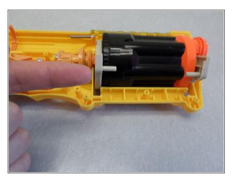
Release the two tan sticks from the holes that they are placed by sliding them upwards.
