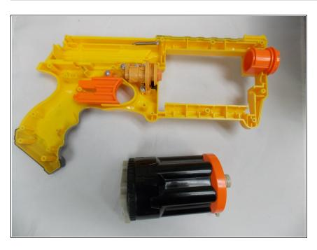
Once you have released the tan sticks, and pulled back on the orange circle, the tension should release the chamber making it easily removable.
