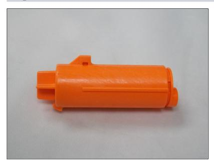
Locate the air plunger in the upper left hand corner of the opened nerf gun. Push back on the spring and carefully pull the plunger toward you to remove it.
