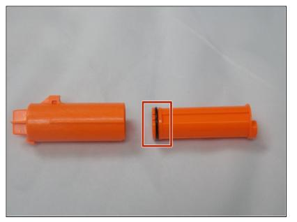
Once you have the air plunger removed, locate the O-Ring by pulling the two pieces of the air plunger apart.
