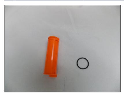
Use a pair of tweezers to remove the O-Ring from the top of the air plunger.
