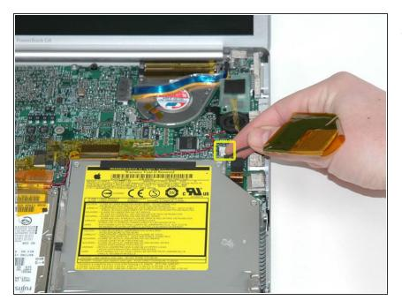
Disconnect the PRAM battery cable from the logic board and pull the PRAM battery out, removing tape as necessary.
