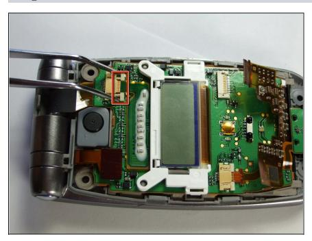
Unlock the minor LCD connector by applying bilateral pressure with tweezers, as shown.
