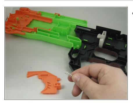
Take the broken spring off of the trigger.
