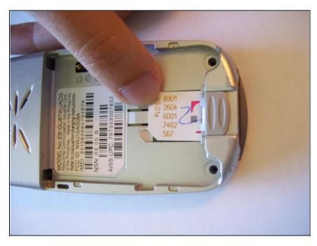
Using your index finger, insert the SIM card into the slot, making sure it's face the right direction.
