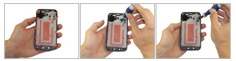
• Use a Phillips 0 screwdriver to remove all 12 Phillips #0 screws.
