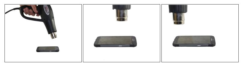
Make sure the battery, the SIM card, and the MicroSD card have been removed. If these components are not removed, they may get damaged when the heat is applied.
