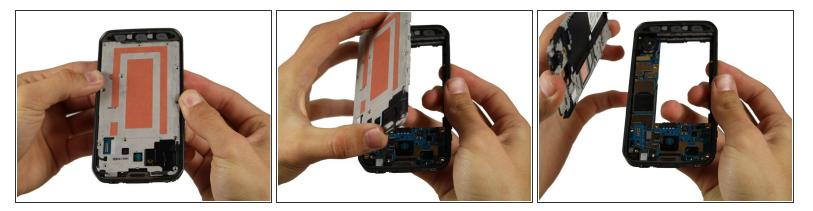
• Push upward from the back side your phone (where the battery should go) to pop out the large gray piece.
