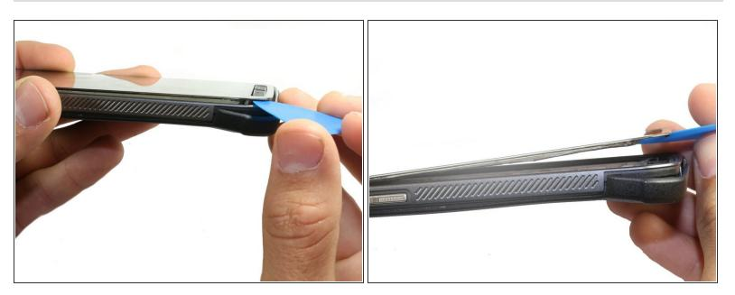
• Using the guitar pick, lift the screen slightly.
