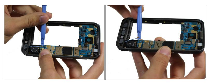
• Use a plastic opening tool to disconnect the the blue wire shown in the picture.
