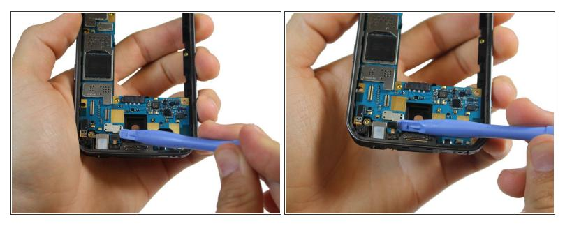
Use your finger or a plastic opening tool to disconnect the proximity/light sensor from the motherboard.
