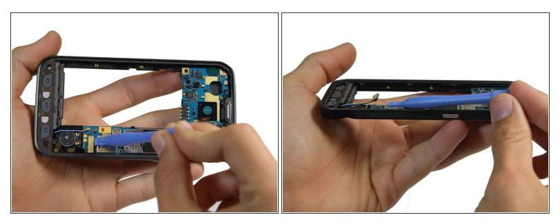
Use your finger or a plastic opening tool to disconnect the 3 button ribbon cable from the motherboard.
