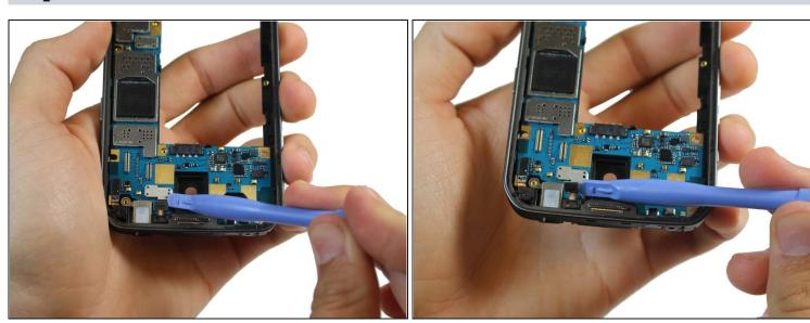
• Use your finger or a plastic opening tool to disconnect the front-facing camera from the motherboard.
