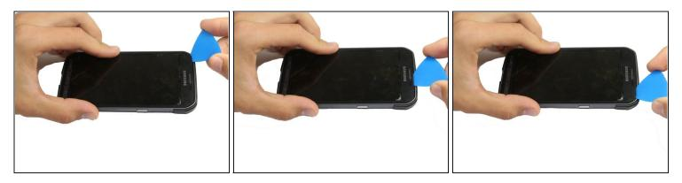
• Use the pick to pry the display by sliding the pick in the direction shown.
