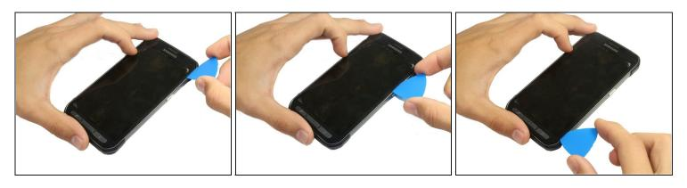
• Use the pick to pry the sides and lower part of the display by sliding the pick through the phone.
