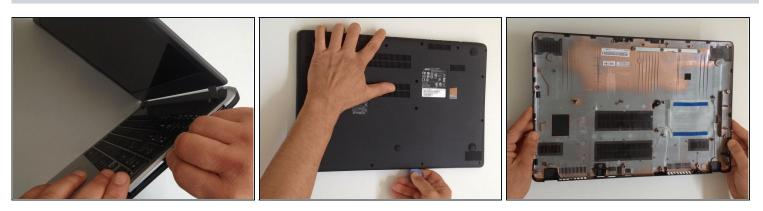
• Starting from the SD Memory Card hole, start prying between the top and bottom cases.
