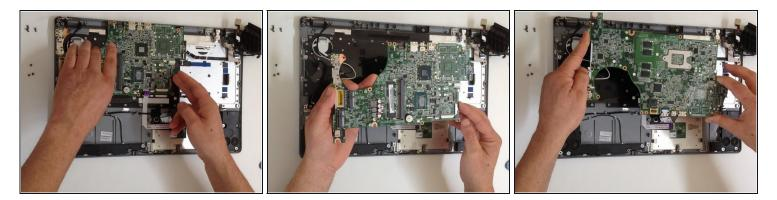
• Carefully remove the the Main board.
