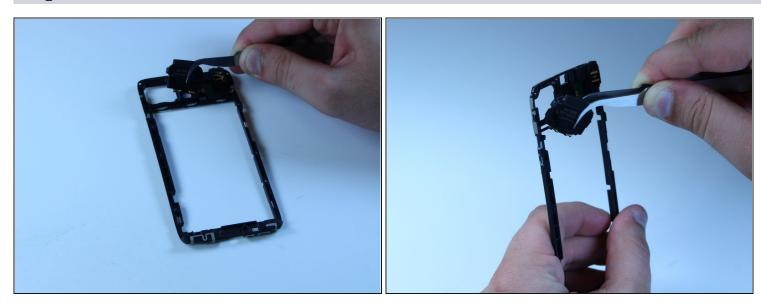
• Use the <u>tweezers</u> to gently push the loudspeaker out of the housing frame.
