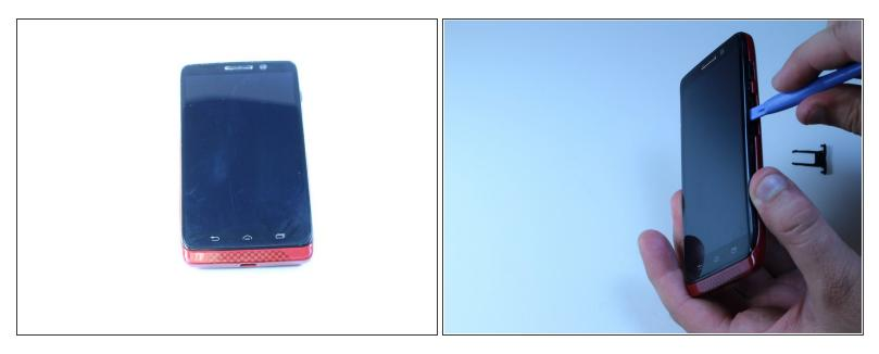
• Pull out the volume keys using the iFixit opening tool.
