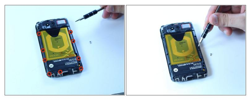
• Use the T5 screw head to unscrew the 9 silver screws from the housing frame. Carefully separate the housing frame from the motherboard.
