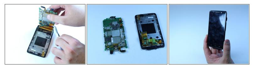
• Carefully use the tweezers to separate the motherboard from the screen.
