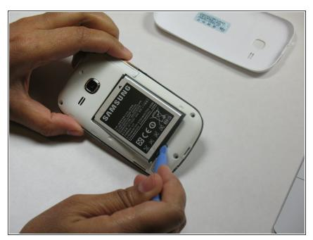
Remove the battery with plastic opening tool
