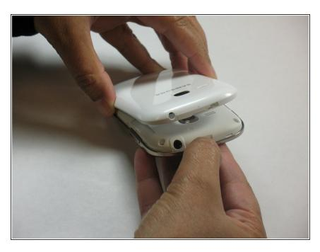
Start by removing the back cover by using your thumbnail to pry the cover off the midframe.
