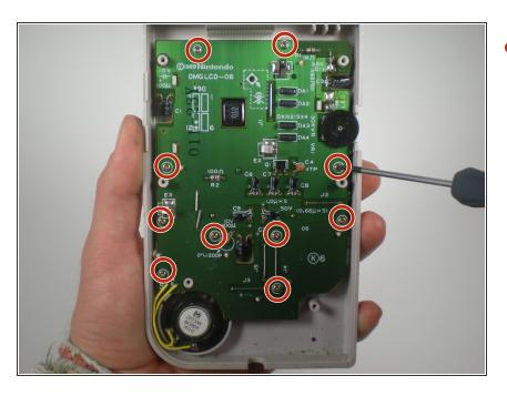
Remove the 10 Phillips #00 screws from the motherboard.
