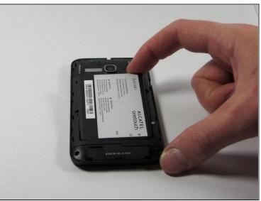
• Place finger in the tab on the top right corner of the battery indicated by a black arrow. With slight pressure, push battery down and out of the slot until the battery is removed
