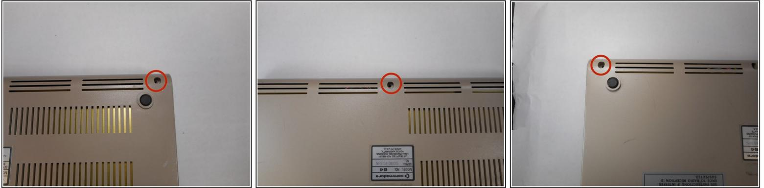
1. Remove three 6.75mm ph2 screw heads from the casing
