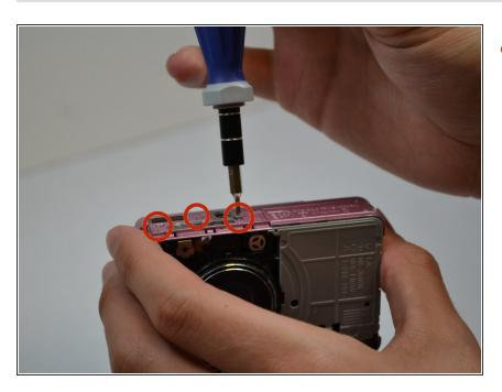
Unscrew the three screws at the bottom of the camera.
