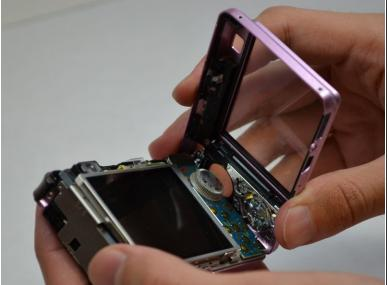
• Using a plastic opening tool, carefully separate and remove the back case.
