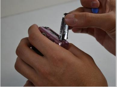
• Using a plastic opening tool, lift and remove the silver piece on the right side of the camera.
