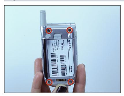
Unscrew all four, 5mm Tri-Wing screws.
