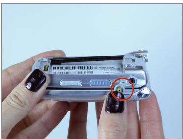
• Pry the back casing off the device using a spudger. Work your way along the edges to completely separate the back casing from the device.
