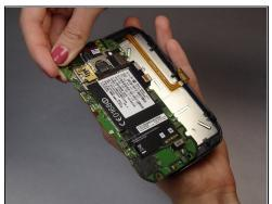
⚠ Be careful when removing the motherboard. The earpiece is connected with small wires and adhesive. Use a thin tool to pry it off before removing the motherboard.
