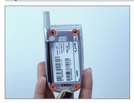
Unscrew all four, 5mm Tri-Wing screws.
