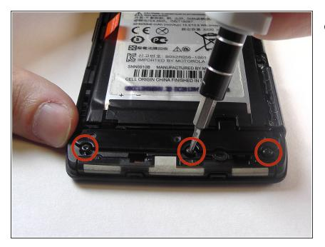
Using the T4 bit piece remove the three black 4.5 mm screws that are located at the bottom of the phone.
