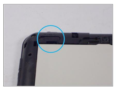
Locate the lock switch, at the top left corner of the device, and adjust to the unlocked position. (from left to right)
