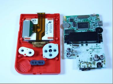
• Grab the black piece protruding from the motherboard, and lift up to remove the motherboard.
