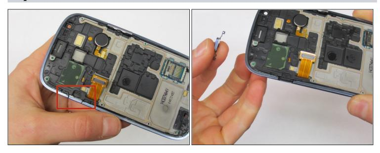
• The power button is connected by two plastic posts, simply lift the button away from the phone using your fingers.
