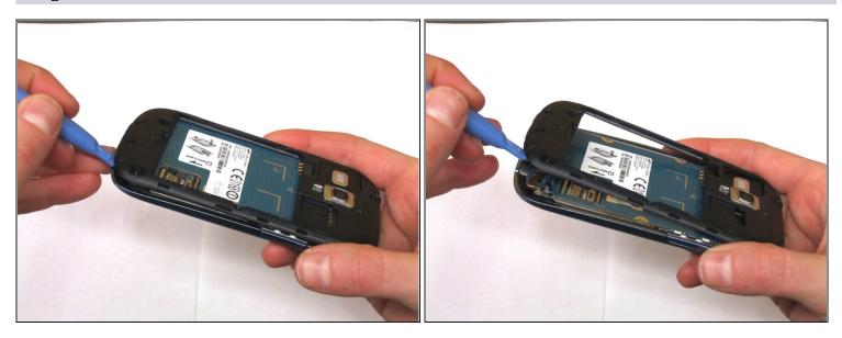
Using an opening tool, gently separate the plastic framing from the phone.
