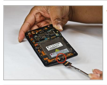
Using a smudger, lift the charger port and replace as necessary.
