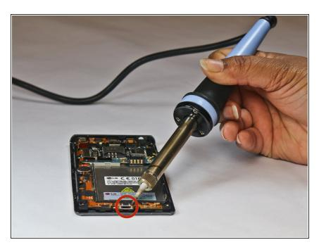
Using soldering iron, loosen the charger port from the bottom of the device.
