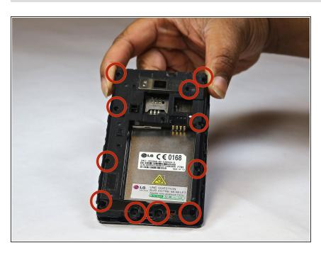
Remove the 12 screws (with the phillips head 000) around frame and near sim and sd cards.
