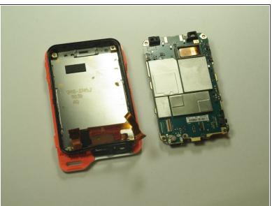
Remove the power strip on the back side of the motherboard.
