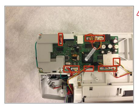
Carefully unplug all of the plugs that are connected to the main motherboard indicating in the picture.
