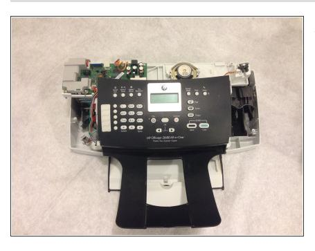
Once the rear plastic panel has been removed, you are ready to replace and repair the necessary parts.
