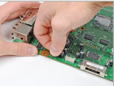
Disconnect the optical drive power and SATA cables from the motherboard.
