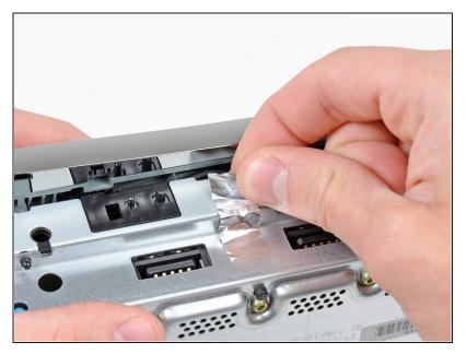
Peel the silver tape securing the optical drive to the metal casing.
