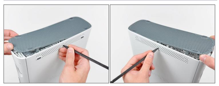
• Repeat the same process to release the two center clips on the bottom vent.
