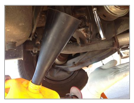
• Before proceeding to the first step of the removal of your tank strainer you will need to drain your fuel tank and remove the main fuel feed line that screws in to the body of the tank strainer. See the rear fuel line replacement guide for guidance on this process.
