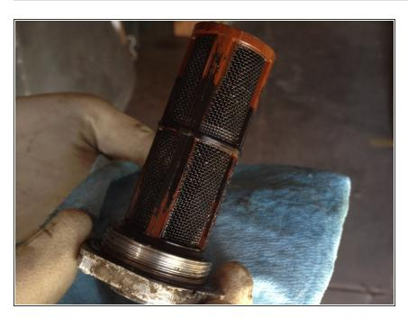
With the tank strainer removed you can inspect it. This one was very clean when removed from the car. It needed little to no cleaning.
