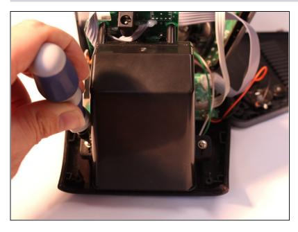
Remove two 9mm screws holding speaker assembly in iP21, using iFixit Phillips #2 bit
